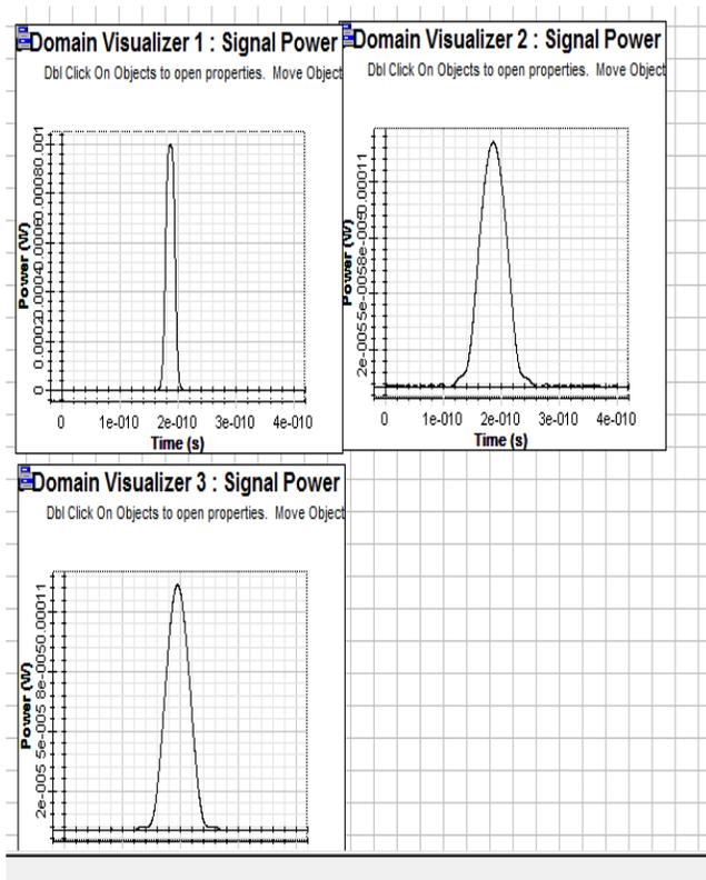
Fig.3 Plot of waveform which shows dispersion loss and compensation at input, middle and the output sides
