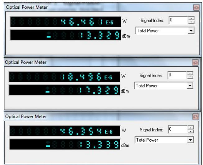
Fig.4 Plot of measured power at input middle and the output side
